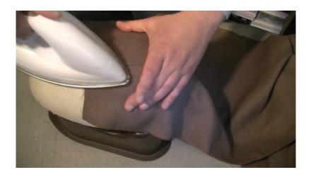
Pressing a dart into a pair of trousers using a tailors ham for shaping in conjunction with the steam iron.
